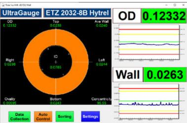
The Total Vu HMI is fully configurable: the operator interface can be as simple as you want or as sophisticated as you need.
