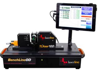
The BenchLinc OD system includes a spring-loaded chuck that accommodates products with diameters down to .001" [25 µm]. It uses a laser micrometer to deliver optimal accuracy by checking sample diameter from multiple angles. Users control the number of measurements per sample and degrees between measurements. These settings are included in recipes for quick, product-specific changeovers and consistent results.
