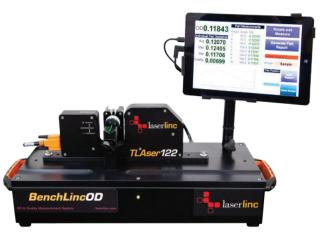
The BenchLinc OD system includes a spring-loaded chuck that accommodates products with diameters down to .001" [25 µm]. The laser micrometer checks sample diameter from multiple angles, for optimal accuracy. Users control the number of measurements per sample and degrees between measurements. These settings are included in recipes for quick, product-specific changeovers.
