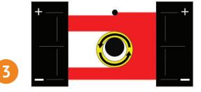
The sample is automatically rotated to multiple positions for measurement. Diameter, ovality and concentricity are displayed and recorded.
