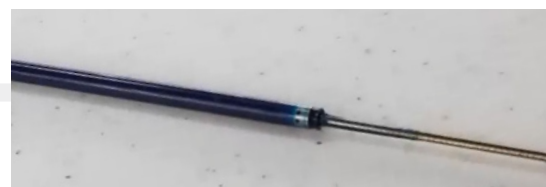
Automated mandrel detection ensures that only the product's OD is collected
