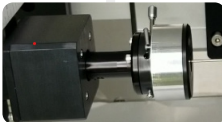
MPR: automated motorized chuck rotates the part to measure up to 360° around the product
