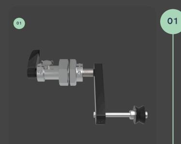
Part Guiding Roller Guides: Supports up to 3 lbs of downward force. Multiple roller guides can be used to distribute the load in both freestanding and tank-mounted configurations.
